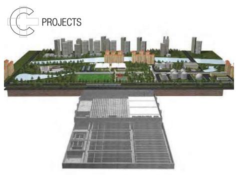
The fully underground multi-layered sewage treatment facility goes 17 metres deep
