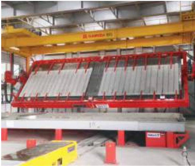
The Banting factory manufactures double walls for even taller buildings
