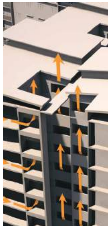
Stack effect allows outflow of hot air
