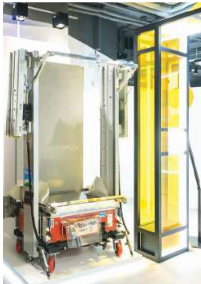
Automatic Wall Plastering Machine
