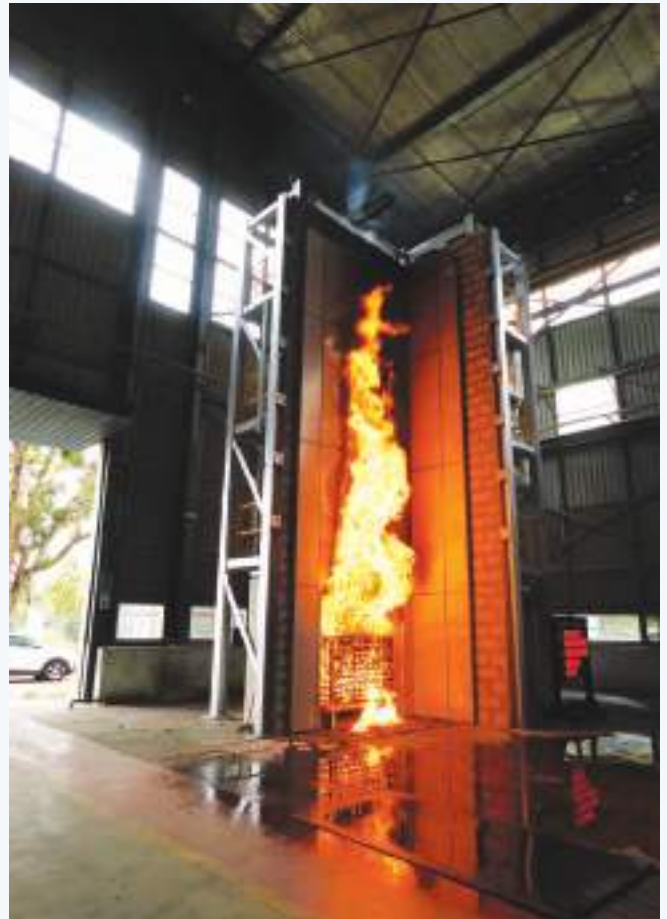
Vitaly's BS8414-1 test conducted @SIRIM Rasa
